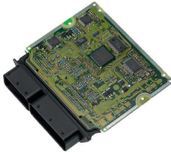
Figure 2.243 Inside an electronic control unit (ECU)
